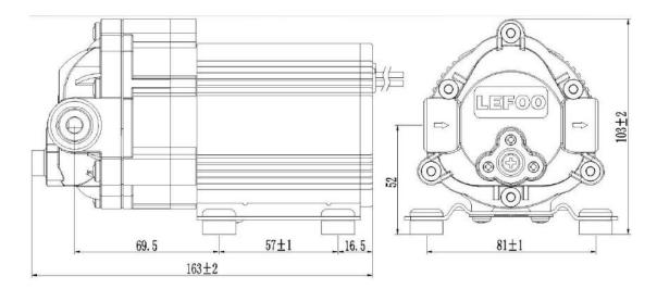
Mounting Dimensions (mm) :LFP2800W-B / LFP21000W-B
