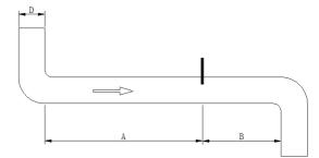
Due to different pipelines and turbulence effects and other factors, depending on the sensor, the wind speed sensor should be installed for multiple position adjustments. It is recommended that the measurement point of the single-point wind speed sensor should be selected at one-third or two-thirds of the pipe diameter, and observes that the measurement result does not jump too much, avoid measuring the pipe wall or pipe center.
