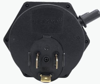
LF31A switches offer pressure, vacuum and differential models capable of sensing very low setpoints, and switching current up to 5A resistive, 2.5A inductive. Designed for use in the HVAC industry, where reliable air proving is critical to both performance and customer safety. The LF31A is a favorite with leading manufacturers of gas-fired warm air furnaces and water heaters.
